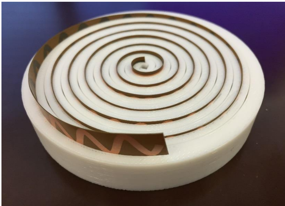
Figure 3.4. Additive manufactured Polycarbonate dielectric with PSA element partially installed.
