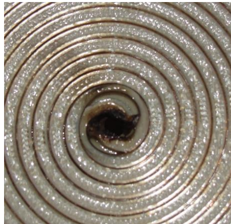
Figure 3.12. Damage incurred during thermal testing with 50 W incident power at 3 GHz.
