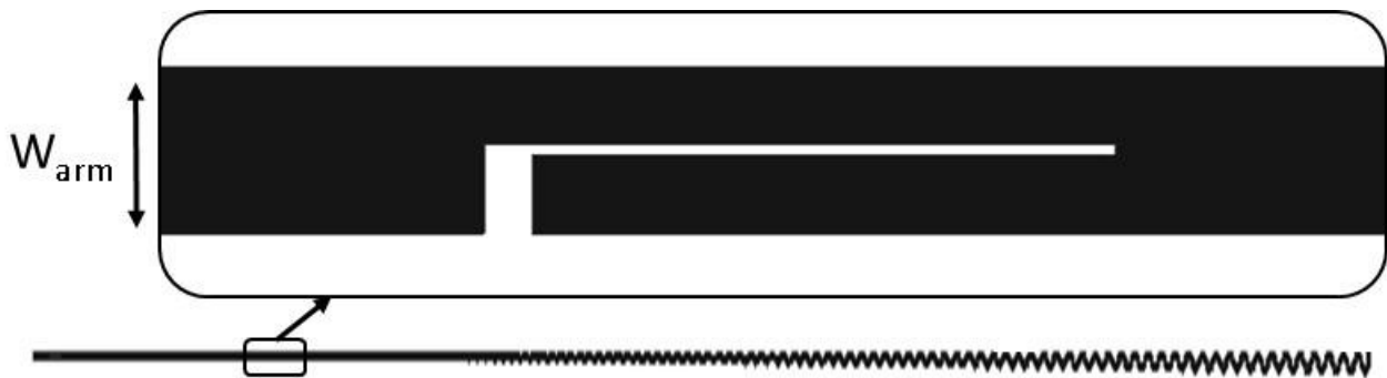
Figure 4.9. Location and configuration of the symmetric spurline filter along the length of the spiral arm.
